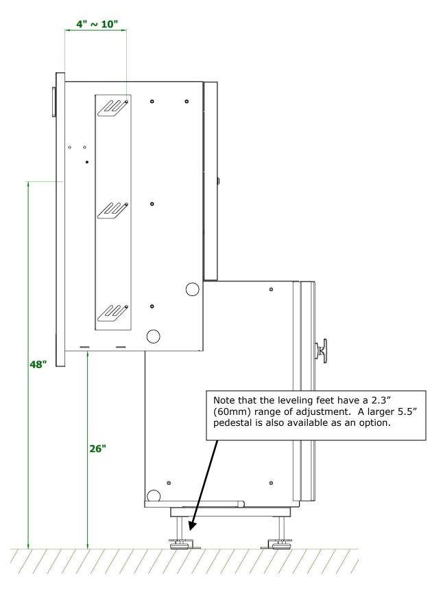
The following shows how to set the hole dimensions so that the machine will have the correct height for ADA compliance.
