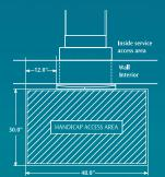
The dimensions shown comply with U.S. Federal ADA guidelines. For installation within the Us., be sue to check statand local guidelines for complete compliance. For non-USA installations, check regulations for the country in which the machine will be installed.
